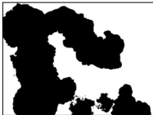
Rust Grade 1-S, 50% Rusted
